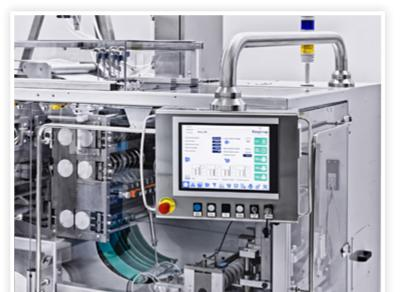
New open-source software & UX navigation widescreen 15"Touchscreen, compatible with ERP software.
